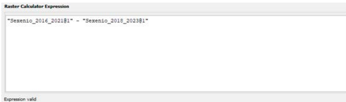
Figure 16. A raster calculator calculation was performed to determine the pixel dynamics between six-year periods.
